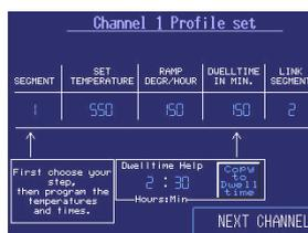
On the profile setting screen, there are four parameters that can be set for each segment. First select the segment you want to set by touching the segment number. The keypad will pop-up and you can select the segment you want to program, from segment 1 to segment 8. Always start your programm in segment number one!
