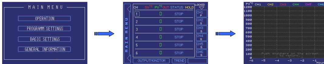
In “Lock mode”, the operator still has the possibility to swap to the all channels trend, by pushing the button “TREND”. Touching the trend screen just anywhere, returns you to the “RUN/STOP LOCK” screen.
