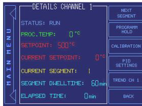
e) To swap to the “DETAIL CHANNEL SCREEN”, you have to touch the blue rectangled programm channelnumber. This means you can see the detail information of all different programmers by touching the corresponding channel.
