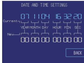
d) On the “DATE AND TIME SETTINGS” page you can set the correct date and time that will be used in the automatic datalogging feature. This will make sure that the correct date and times are used in the .csv file that you can create on the “COPY DATA” page. The blue numbers are the current settings, the white settings are the new settings. Just touch the white numbers, and type in the desired date and time. The new values are active immediately.
