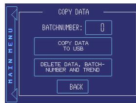
e) Push the “COPY DATA” button to enter the “COPY DATA” screen. A batchnumber can be set, that will be used as a filename when copying the data to your USB stick. Of course, make sure your USB stick is connected. After copying the .csv file to your USB stick by just pushing the “COPY DATA TO USB” button, you can delete the logfile by pushing the “DELETE DATA” button for 3 seconds.
