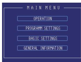
a) Push the “PROGRAMM SETTINGS” button to swap to the Profile Setting menu, where you can start setting the profile of channel number 1.
