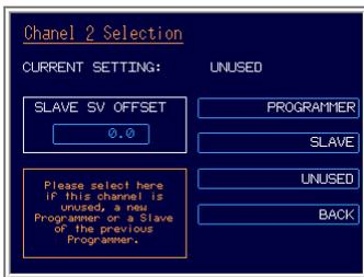
On the “Channel selection screen” you can select each channel to be a programmer, slave of the previous programmer or unused, by pushing the corresponding button. You can go back to the previous channel at any time, by pushing “BACK” button.
