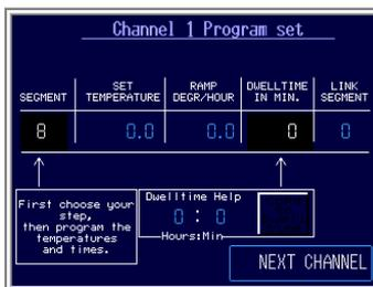
On the profile setting screen, there are four parameters that can be set for each segment. First select the segment you want to set by touching the segment number. The keypad will pop-up and you can select the segment you want to program, from segment 1 to segment 8. Always start your program in segment number one!
