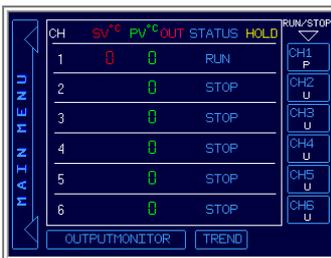
To run or stop a program, toggle the corresponding programmer channel button for *one* second. The one second delay on this button is to prevent a operator from switching a program by accident. The slave(s) that belong to this programmer will automatically follow the run or stop status of the programmer.
