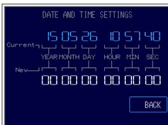
On the “DATE AND TIME SETTINGS” page you can set the correct date and time that will be used in the automatic data logging feature. This will make sure that the correct date and times are used in the .csv file that you can create on the “COPY DATA” page. The blue numbers are the current settings, the white settings are the new settings. Just touch the white numbers, and type in the desired date and time. The new values are immediately active.
