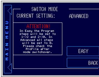
To switch to a different mode (easy or normal) go to the “switch easy/normal” menu.
