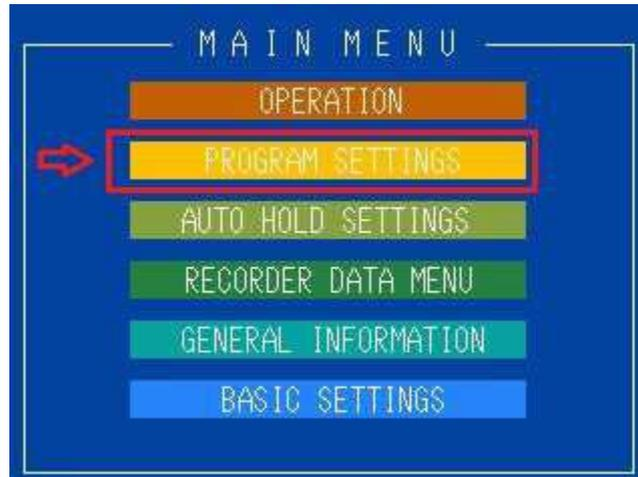
Push program settings for setting the correct type of channel. Remember that channel 1 is always a programmer.
