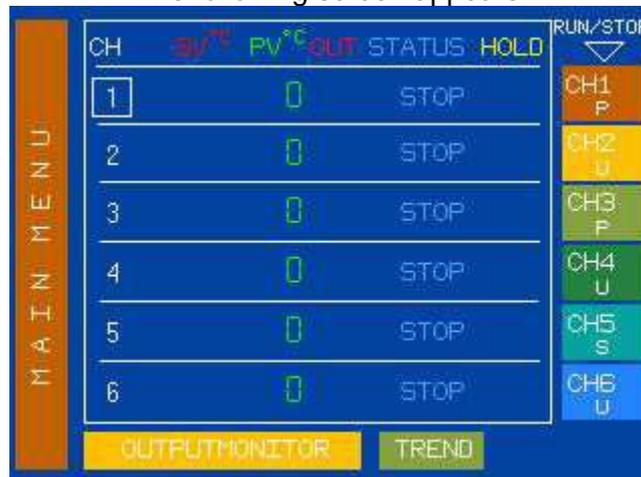
This shows a situation with channel 1 as a programmer [ 1 ] is boxed and the letter **P** under **CH1** on the right side.
