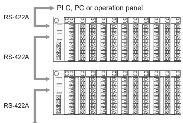
Up to 16 units (Max. 320 loops) are available when connected to a RKC touch screen operation panel, PLC or a host computer.
